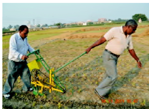
Sowing with the help of No-Till Drill with two manpower
